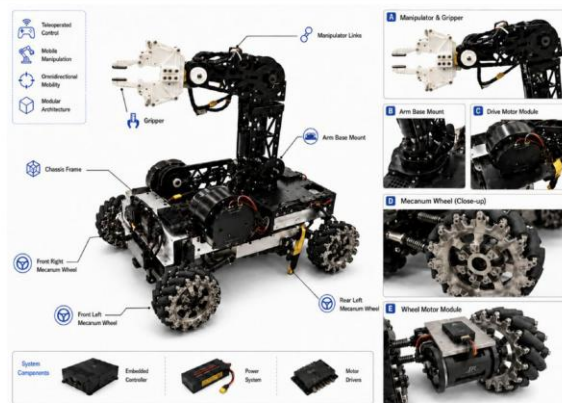
Mechanical/electrical design details (real build)
