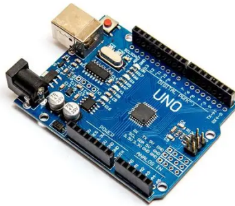
Figure 2: Arduino Uno R3 controller board used as the central embedded controller in the final prototype [5].
