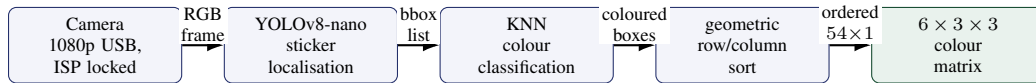
Figure 7: Decoupled vision pipeline. Locking the camera’s auto-exposure and white balance stabilises RGB values when the white 3D-printed arms enter the field of view; YOLOv8 then performs class-agnostic sticker detection, KNN assigns a colour to each bounding box, and a geometric sort emits the 6 \times 3 \times 3 matrix consumed by the Kociemba solver.
