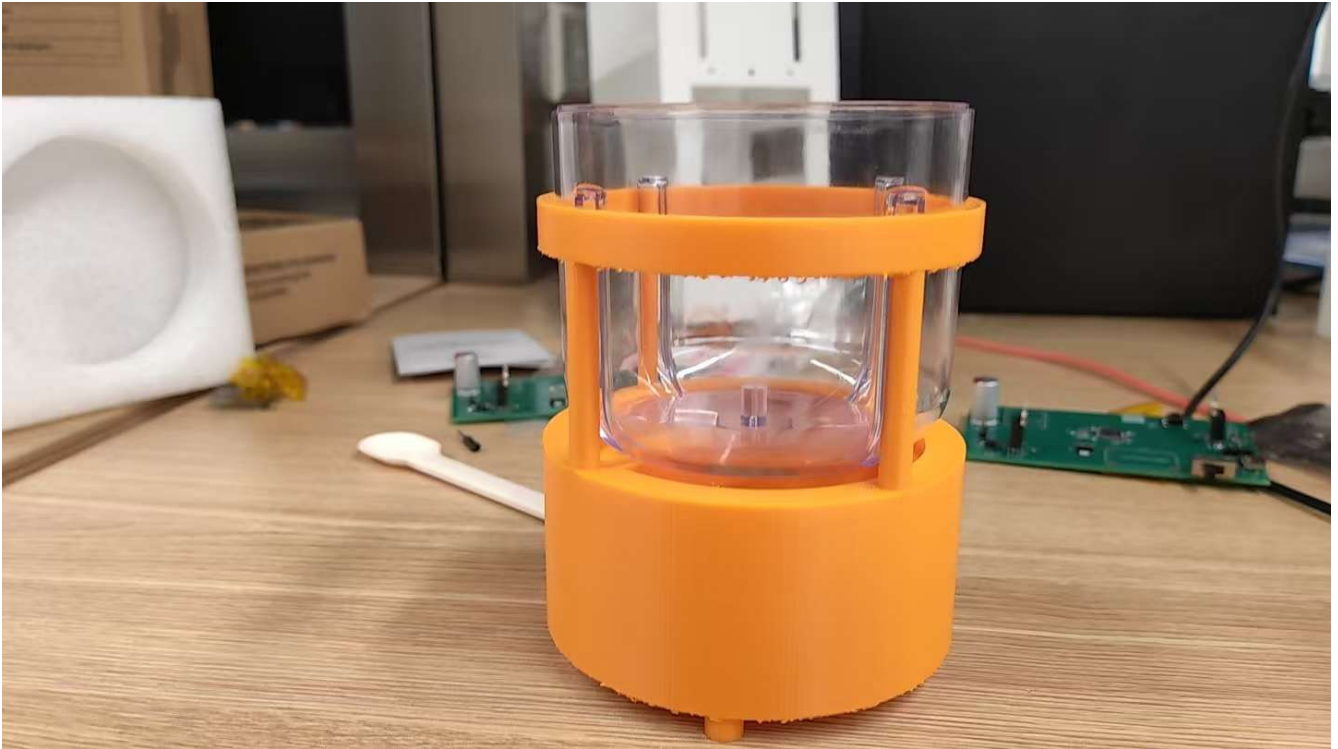
Figure 9. Physical stirring subsystem.
