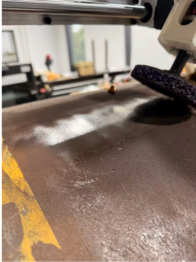
Figure 12: Rust-removal test surface used for end-effector verification.
