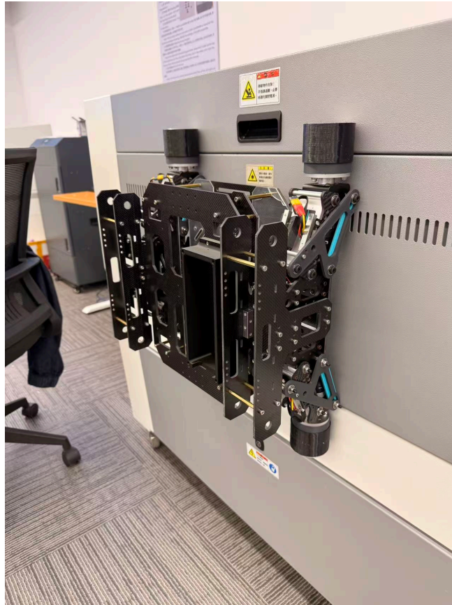
Figure 11: Assembled magnetic-wheeled robot used for adhesion and locomotion verification.
