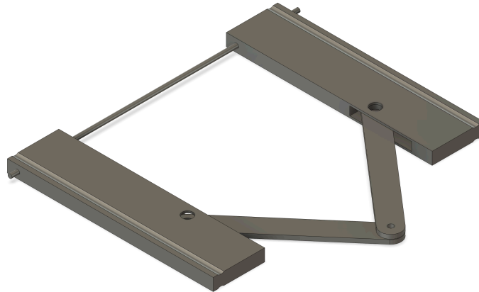
Figure 2.3: The linkage deployment mechanism and guide rails.
