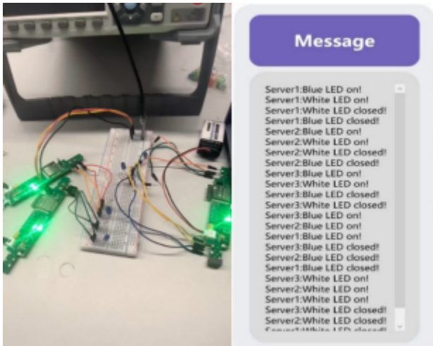
Figure 7. Testing setup for Wi-Fi control module showing (a) experimental test and (b) feedback in the user interface.
