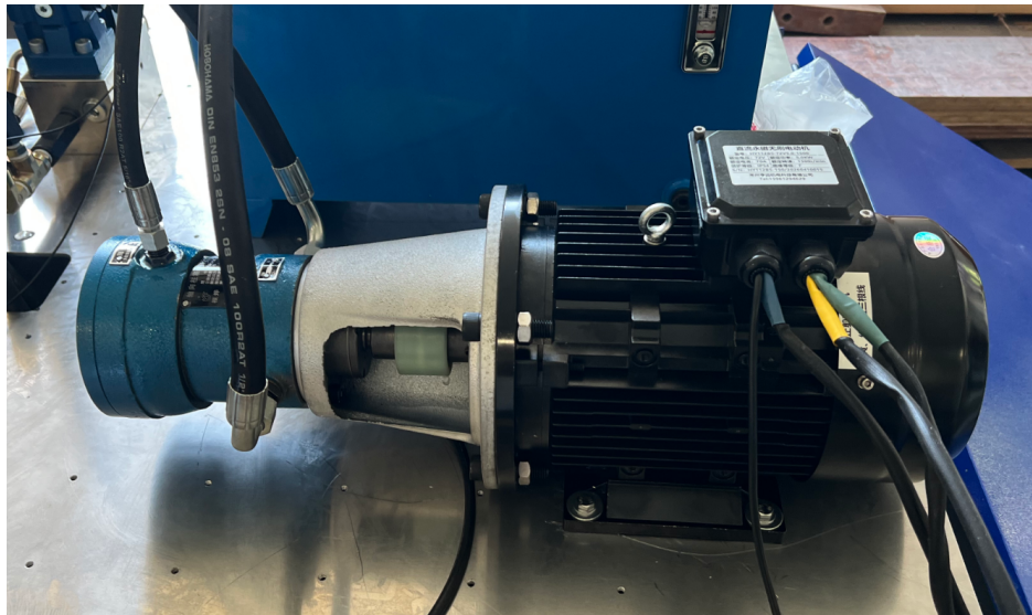
Figure 5: Brushless DC motor and hydraulic pump assembly. The motor converts electrical drive power into mechanical rotation, and the pump converts the motor output into hydraulic pressure and flow.
