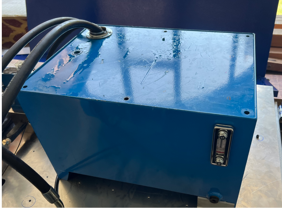
Figure 6: Hydraulic oil reservoir mounted on the vehicle platform. The reservoir stores the hydraulic fluid and provides the return path for the hydraulic circuit.
