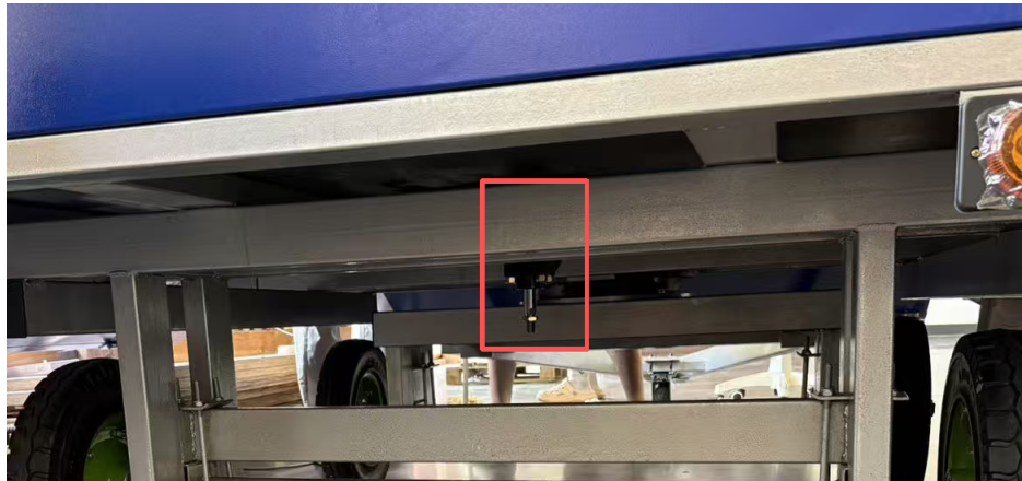
Figure 8: Hydraulic cylinder mounted under the vehicle platform. The cylinder is installed below the frame so that its linear motion can be transferred to the impact or drill-bit end while remaining mechanically supported by the vehicle structure.
