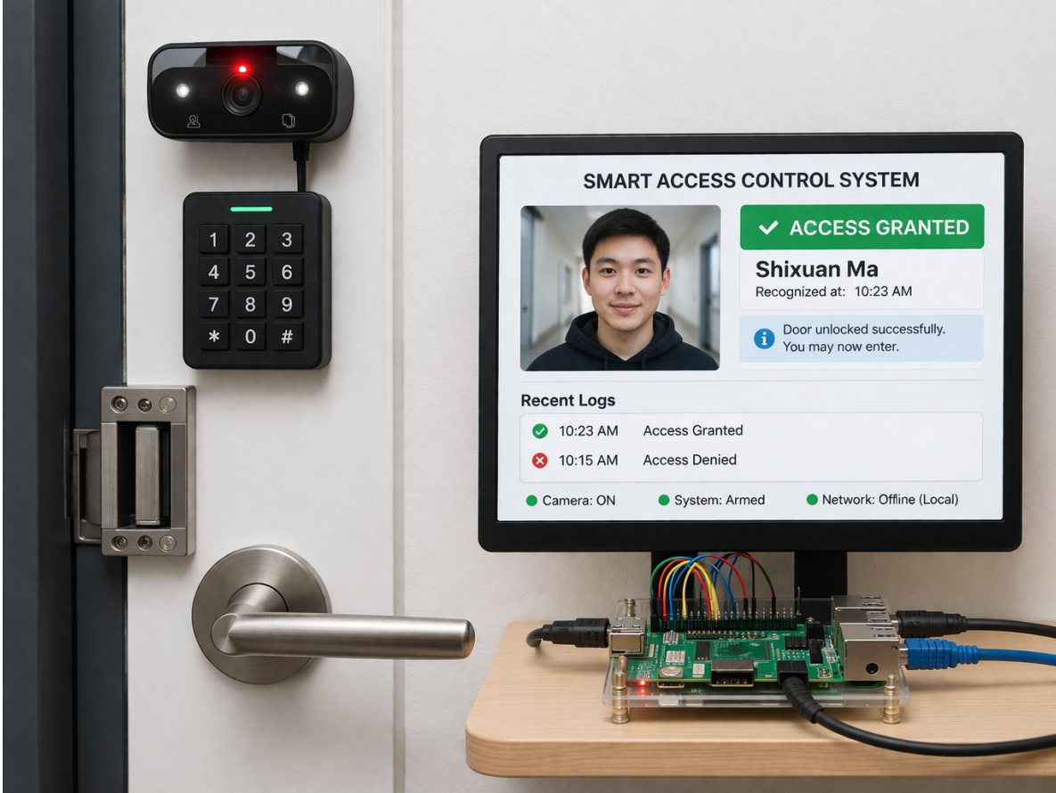
Figure 1: Prototype implementation of the smart biometric access control system, including the door-side sensing unit, keypad, electronic door lock, Raspberry Pi platform, and monitoring display.
