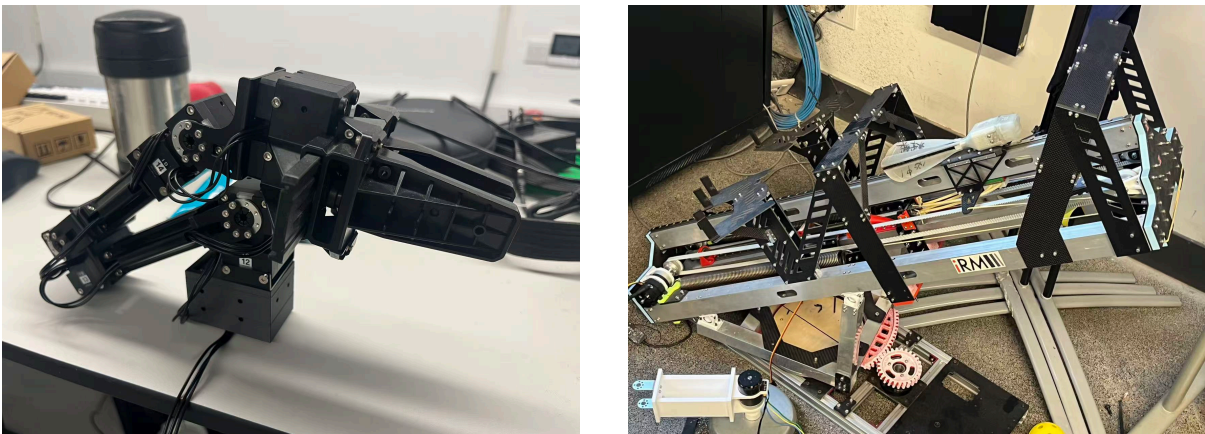
Figure 2: Physical prototypes of the operational system: the multi-axis robotic arm with custom gripper (left) and the friction-wheel launching mechanism (right), demonstrating the hardware utilized for the autonomous staging and firing sequence.
