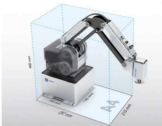
Figure 4: Candidate tabletop robotic arm and its representative workspace.
