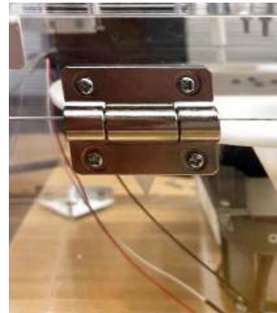
Figure 23: Hinge Connection between Lid and Enclosure
