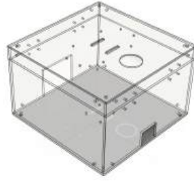
Figure 21: CAD model of the lower acrylic protective enclosure
