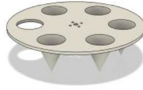
Figure 16: CAD of the Rotating Pill Tray
