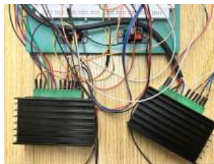
Figure 20: TB6600 Stepper Motor Controllers Connected to the Breadboard System
