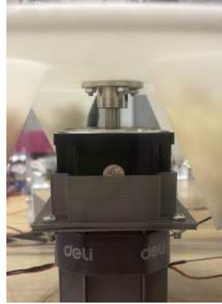
Figure 19: Flange Coupling to Stepper Motor Shaft
