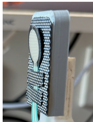
Figure 7: FSR Sensor Installation on Gripper
