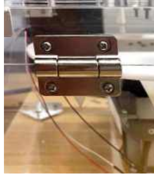
Figure 24: Hinge Connection between Lid and Enclosure
