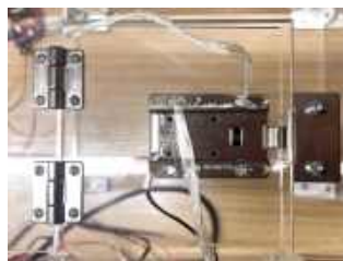
Figure 34: Real Implementation of the Electromagnetic Locking Door
