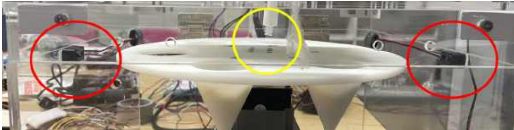
Figure 31: Infrared Break-Beam Sensor Positioned Along the Nozzle's Vertical Path for Pill Presence Detection
