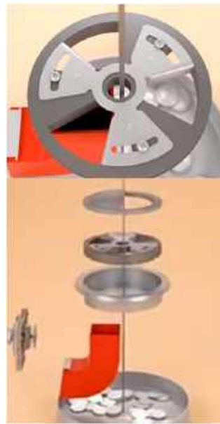
Figure 4: Alternative Design: Gashapon-Style Adjustable Dispensing Mechanism
