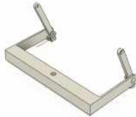
Figure 27: CAD of the Linkage-to-Bracket Dowel Pin Connection
