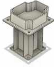
Figure 18: CAD of Stepper Motor Mounting Assembly
