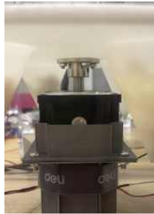
Figure 20: Flange Coupling to Stepper Motor Shaft
