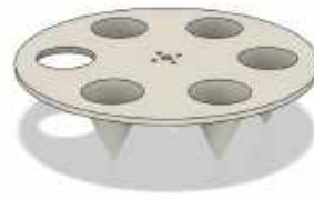
Figure 17: CAD of the Rotating Pill Tray
