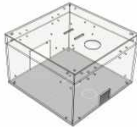
Figure 22: CAD model of the lower acrylic protective enclosure
