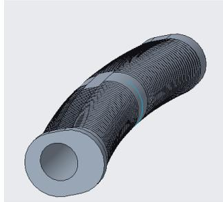
Figure 2: 3D-printed stator spine insert for shaping the flat stack to match the rotor curvature
