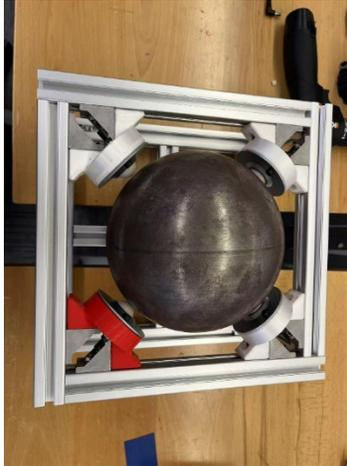
*Figure 7: Top-down view of the rotor support assembly*
