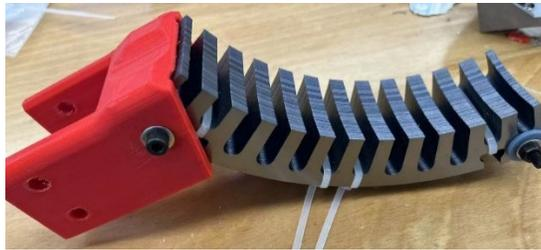
*Figure 8: Assembled stator module showing lamination stack, curvature insert, and mounting bracket*
