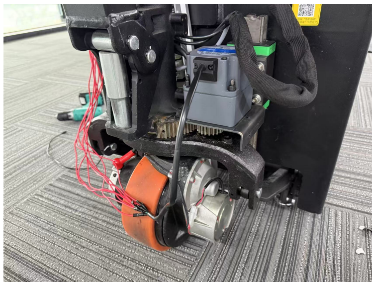
Figure 15: Side motor and gear couple installation
