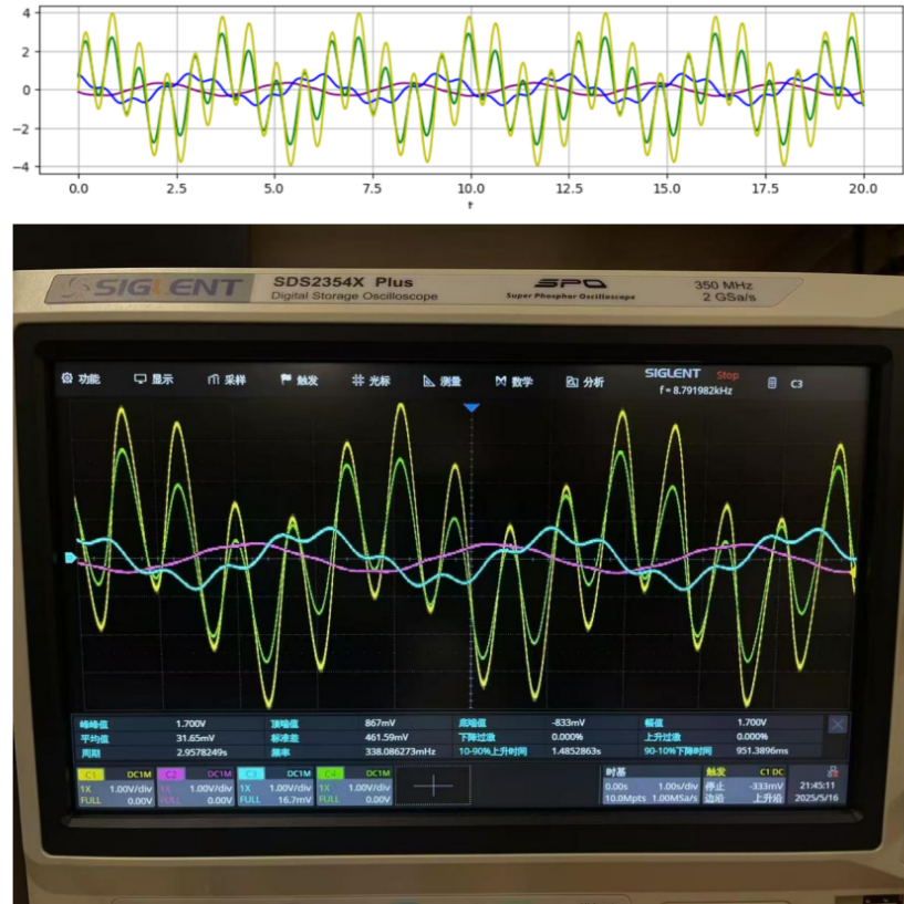
Figure 25: Top: Simulated waveform with Python; Bottom: Measured analog waveform with oscilloscope for composite wave input
