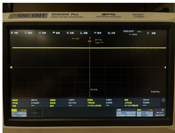
Figure 18: +5 Power Supply by Stable Power Supply
