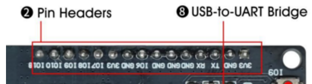
Figure 7: General Purpose Input/Output
