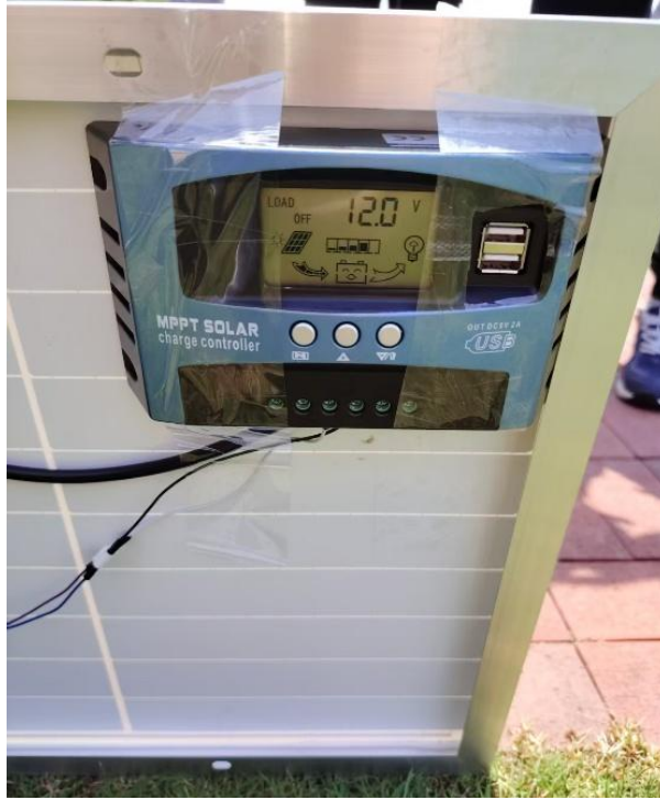
Figure 4.2 MPPT displays the operating voltage within the normal range under the sun, verifying the normal operation of MPPT as expected.
