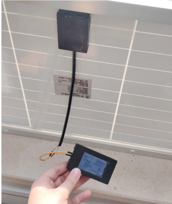
Figure 4.1 The electrical instrument successfully detected that the solar panel outputs 18V, verifying that the solar panel is working properly as expected.
