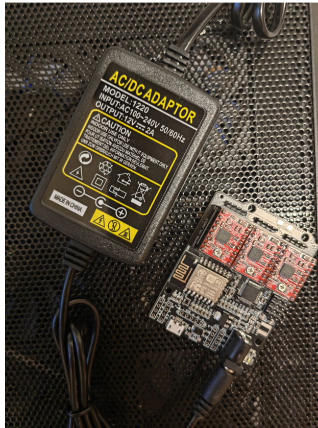
Figure 9: Integrated PCB and AC/DC Adaptor
