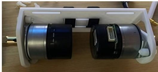
Figure 11 Motor Attached on the Inner Structure
