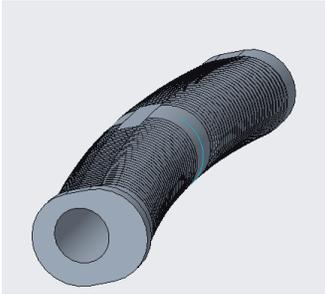
Figure 2: 3D-printed stator spine insert for shaping the flat stack to match the rotor curvature; includes a lip for axial preload.
