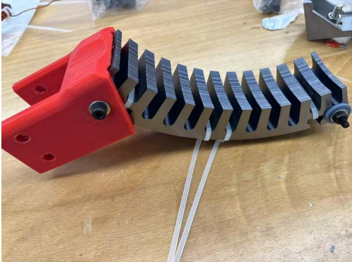
Figure 8: Assembled stator module showing lamination stack, curvature insert, and mounting bracket
