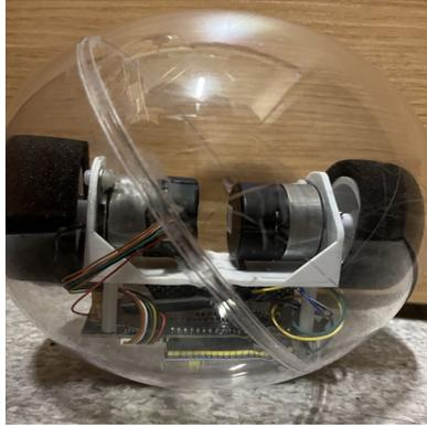
Figure 9 Overview of the ATV Spherical Motor
