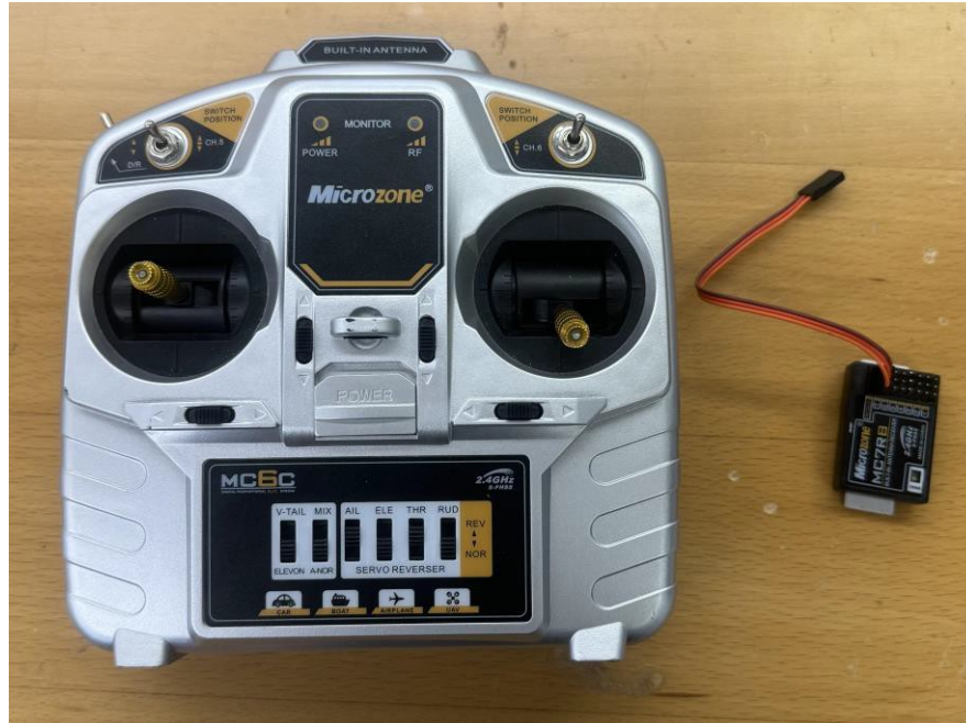
Figure 9: Microzone MC6C Remote Control and MC7RB Remote-control Receiver
