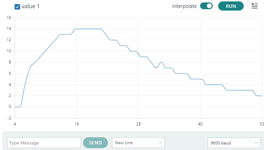
Figure 3.1 Tested Signal in Arduino with x-axis is the time and y-axis shows voltage*5/1024
