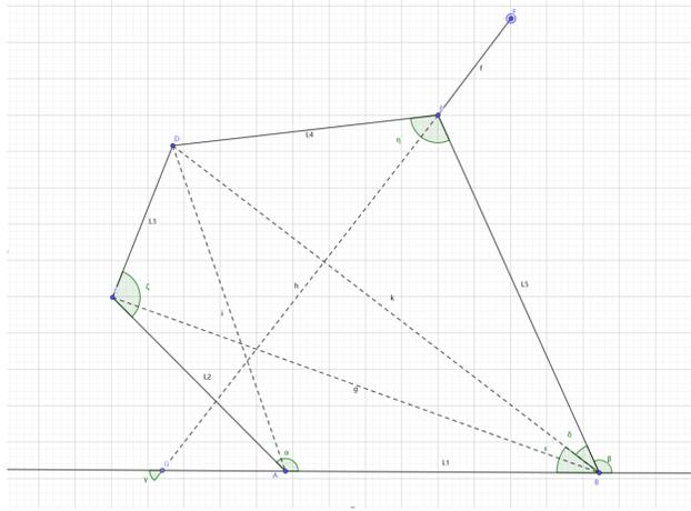
Figure 15: Diagram of five-bar linkage
