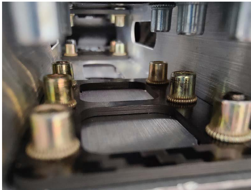
Figure 2.20 Rivet nut in aluminum tube
