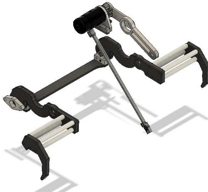
Figure 2.22 The towing rescue mechanism
