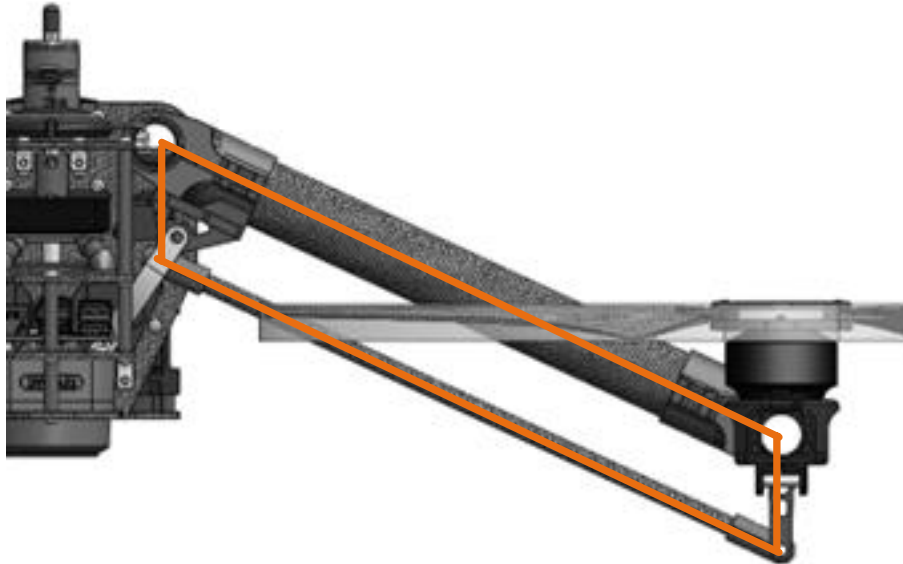
Figure 4 Parallelogram links to keep parallel thrust
