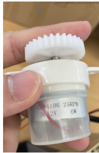
Figure 27: The DC motor with a geared head, designed for low-speed, high-torque brewing. 25 RPM, DC12V and 6W. We need to buy some similar motor.
