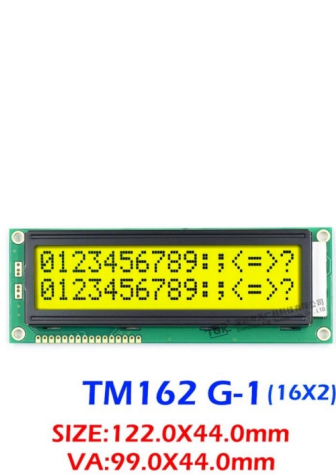
Figure 17: LCD1602 Outside view
