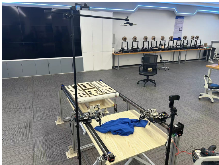
Figure 2.12: Structures of hanging camera(Two black camera stands)
