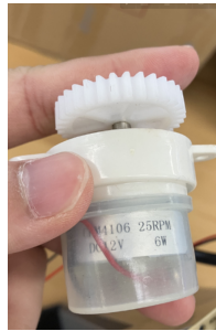
Figure 19: The DC motor with a geared head, designed for low-speed, high-torque brewing. 25 RPM, DC12V and 6W. We need to buy some similar motor.
