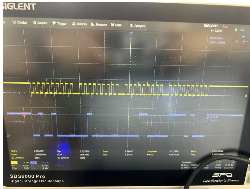
Figure 16 IIC interface measurement by oscilloscope
