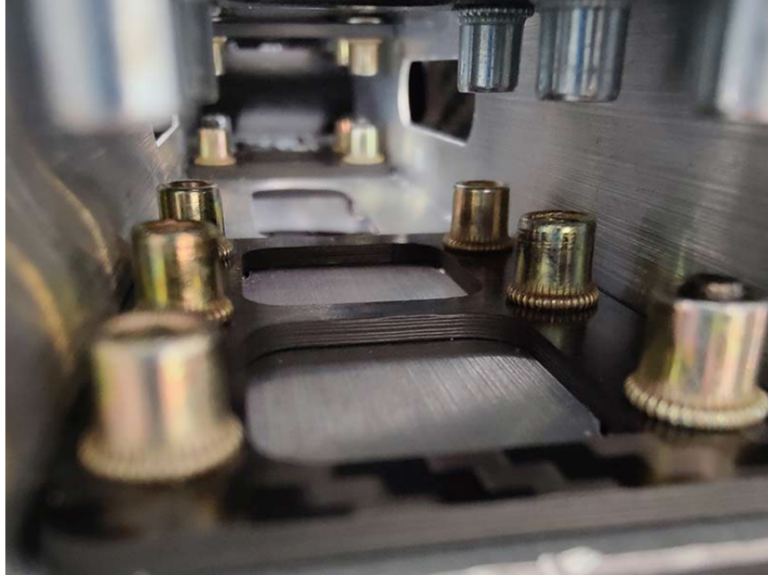
Rivet nut in aluminum tube
