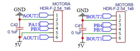
Figure 13: Motor Encoder Interface
