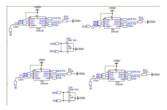
Figure 12: Motor drive circuit
