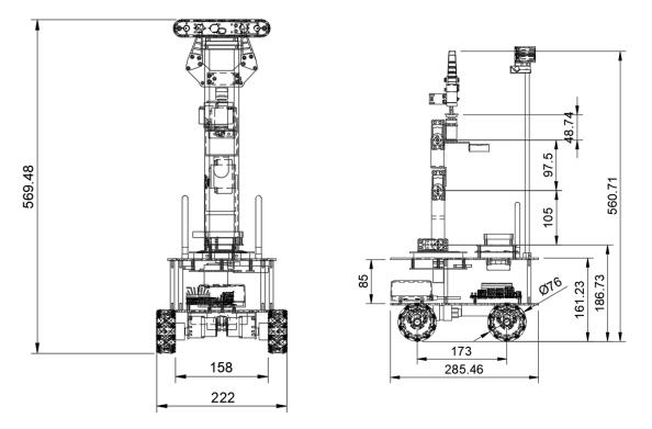
Figure 3: Dimensions of the car
