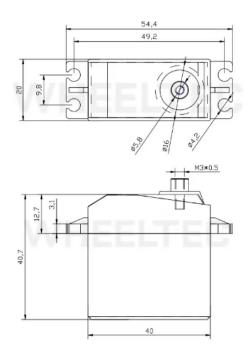
Figure 8: Dimensions of servo
