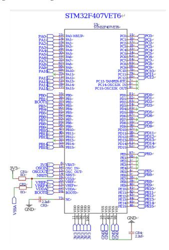
Figure 11: STM32F407VET6 Main Control Board Layout
