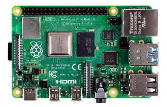
Figure 15: Raspberry Pi 4 Model B
