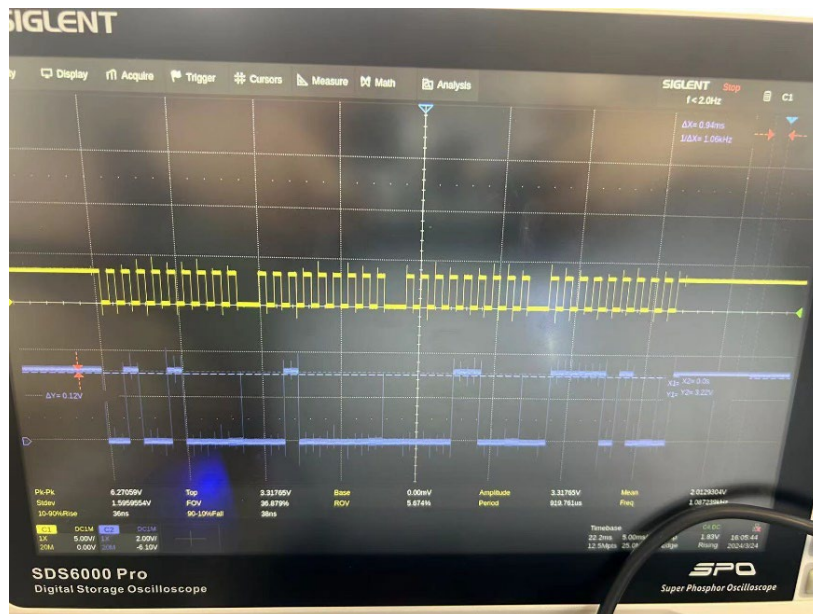
Figure 11 IIC interface measurement by oscilloscope
