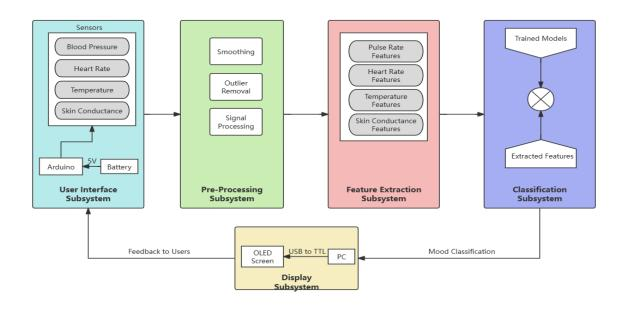
Figure 2: Block Diagram
