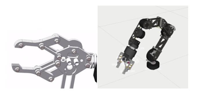
For the material, we will use PLA and use 3D printing technology to print all parts For the arm joints, we plan to use Xiaomi's Cyber Gear motors and KP035 bearing to achieve the movement of the robotics arm.
