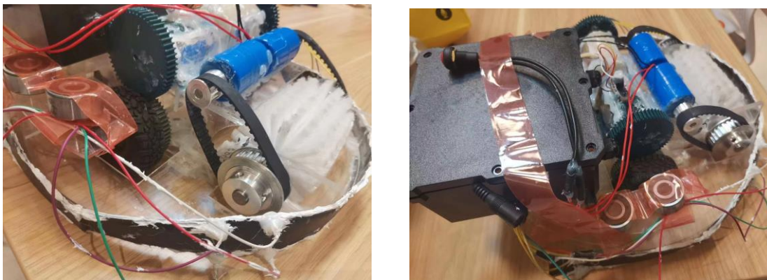
Fig. 29. Waterproofing of pressure sensor and circuits
