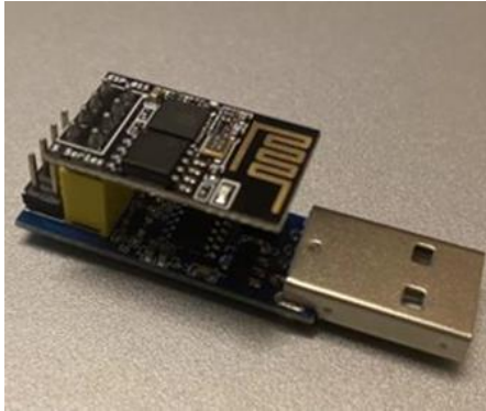
Fig.18. CH340C Connected with ESP8266
