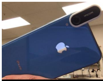
Figure 21. Figure shows the TipScope product, a commercialized brightfield microscope, and how it is used with a smartphone.
