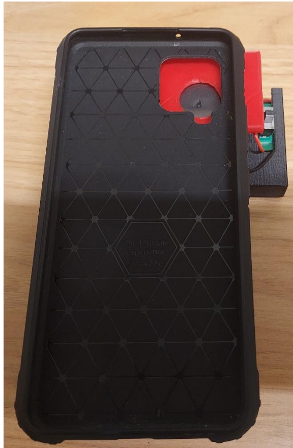
Figure 22. Figure shows how a smartphone will be placed (user hands-free) on Xie's system.
