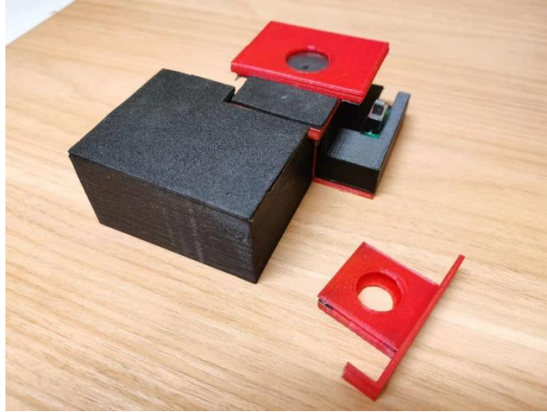
Figure 22. Figure shows the final, 3D printed product designed by Feifan, Xie, where the TipScope, PCB and filters are enclosed within the casing.
