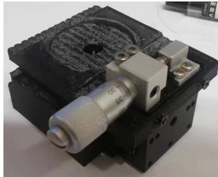
Figure 8. Figure shows the assembled view of filter cover, sample box and camera box with the optical translation stage attached on the side.
