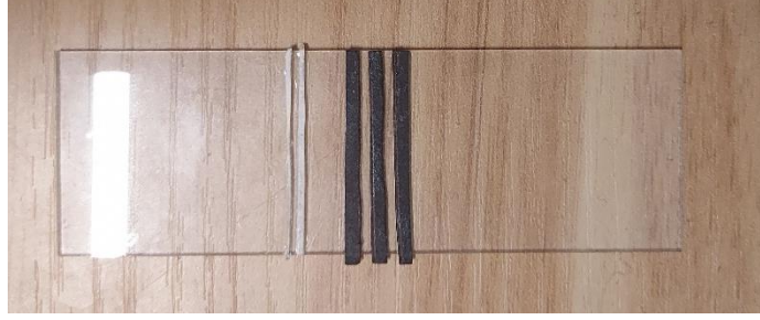
Figure 12. Figure shows a simple calibration tool we used to verify the magnification of the microscope. The black paper strips are 1 mm wide whereas the white paper strips are 0.5 mm wide.
