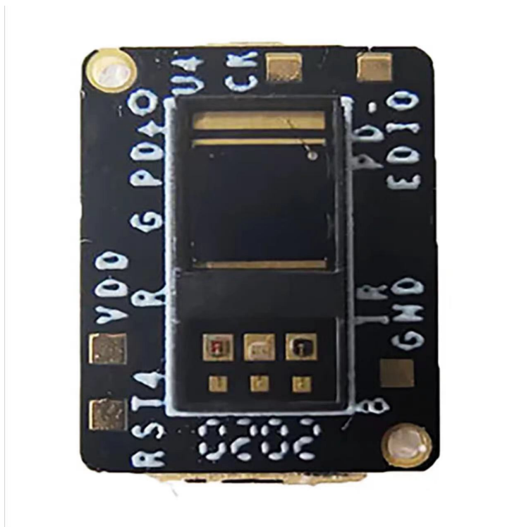
Figure 19: The Vital Sighs Monitoring Chip MQ-R-12 pictorial graph.
