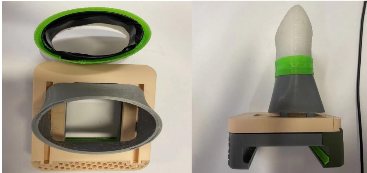
Figure 20 Final mechanical system
