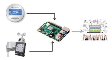
The whole system consists of four parts: a smart meter, a set of weather sensors, a concentrator and a data processing and forecasting terminal. The control computer could be a raspberry PI or some other electronic device. Finally, the data processing terminal can forecast through the obtained power load data and weather data.
