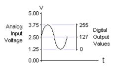
**Digital output:** stream of bytes in range 0 to 255 and scaled approximately such that a 1.25 V input generates a 0 output, and 3.75 V input generates a 255 output.
