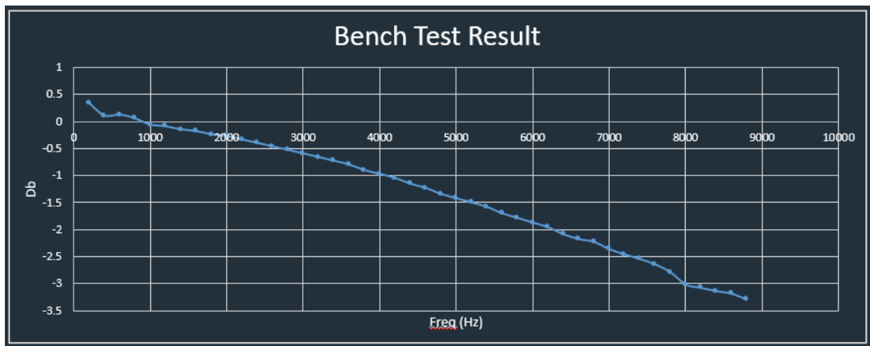
Figure 16. Low-pass filter bench test result
