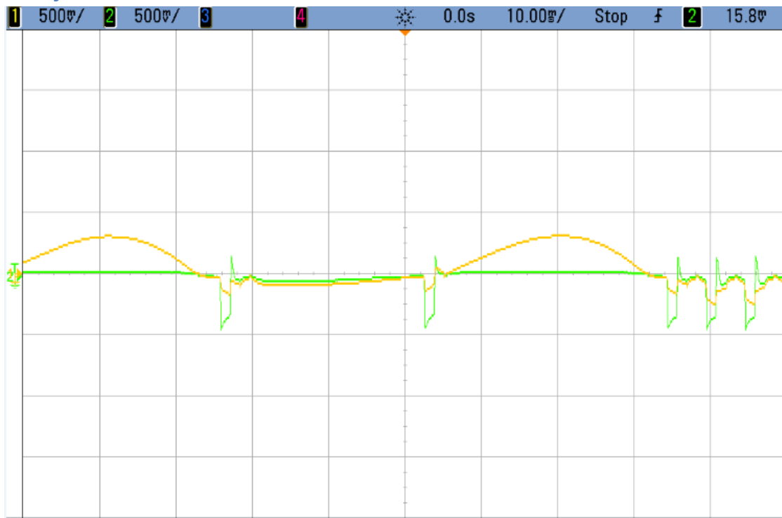
Figure 14 Signal across voltage source (yellow) 17 Hz, 600mVPP vs Voltage output of rectifier (green) .25mV DC
