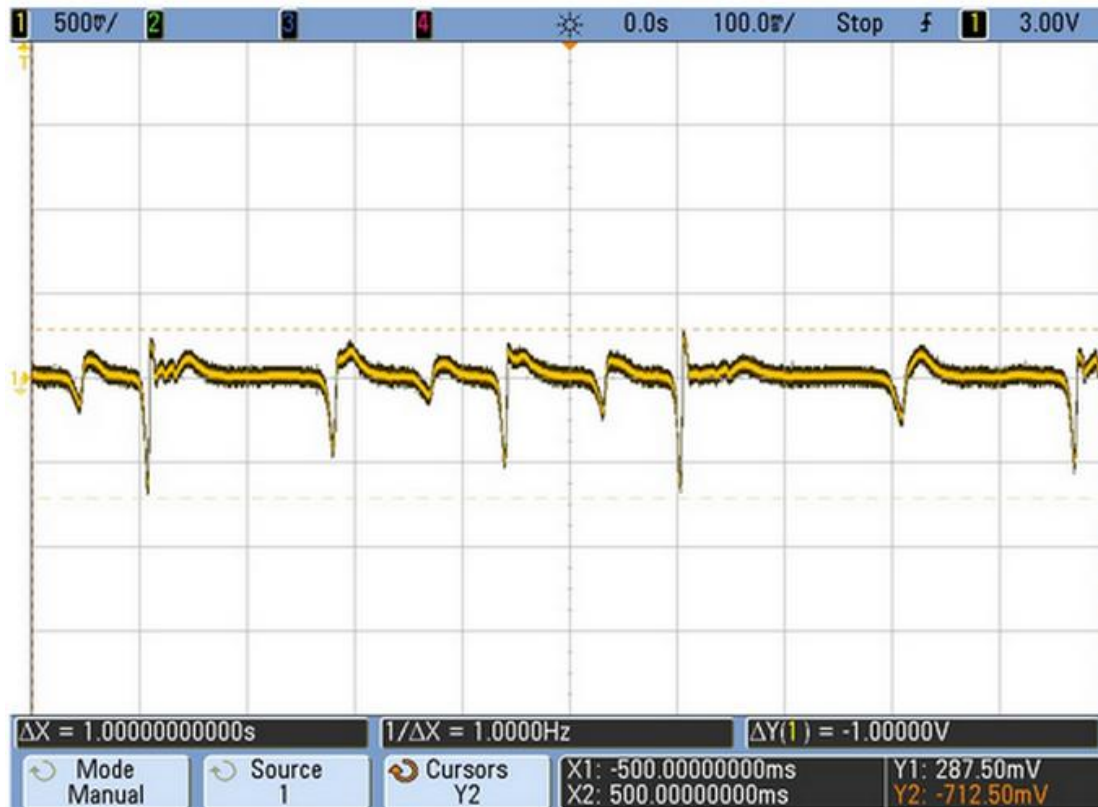
Figure 10 Output from Magnetic Generator
