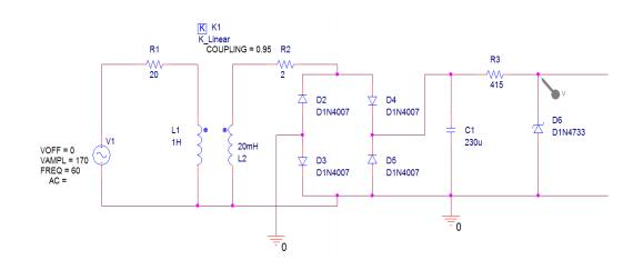
Since the lowered voltage still stands at  $15V_{rms}$ , and the desired voltage is 5V, we employ a regulator, in this case a zener diode in series with a resistor. We use 1N4733 for the zener diode, which provides us with 5.1V zener voltage. To obtain the resistance required to achieve our goal, we calculate it as follows:
