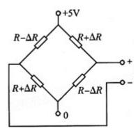
Assume we have the relationship between pressure and resistance R=kP(k is constant) then  $\Delta R=k\Delta P$  so the output voltage of the bridge should be ((R+ $\Delta R$ )/2R-(R- $\Delta R$ )/2R)\*U =  $\Delta R/R*U=k*\Delta R/R*U$ . If we set R1//R4 = R2//R3 and R6//R7=R5, we will get our output voltage Uout= $k*\Delta P*U/R*R3/R2*R7/R6$  which will be sent to our microcontroller.
