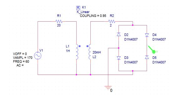
To rectify the alternating current, we intend to take advantage of the feature of diodes. Here, we use the bridge rectifier since it is more efficient than the half-wave circuit or the center-tapped full-wave circuit. Specifically, we use four 1N4007 diodes, from Vishay Semiconductor Diodes Division, to realize that purpose. Since the current can only go under forward-biased condition, the output current will be positive as desired.
