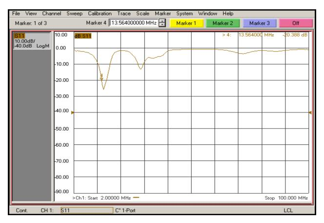
Frequency sweep analysis between 2-100 MHz; return loss of approximately -20dB at 13.56MHz!
