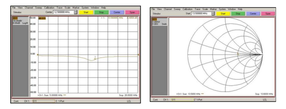
There is a resonant frequency very close to 13.56 MHz; the Smith Chart shows that the antenna and matching network are tuned almost exactly to 50 ohms.
