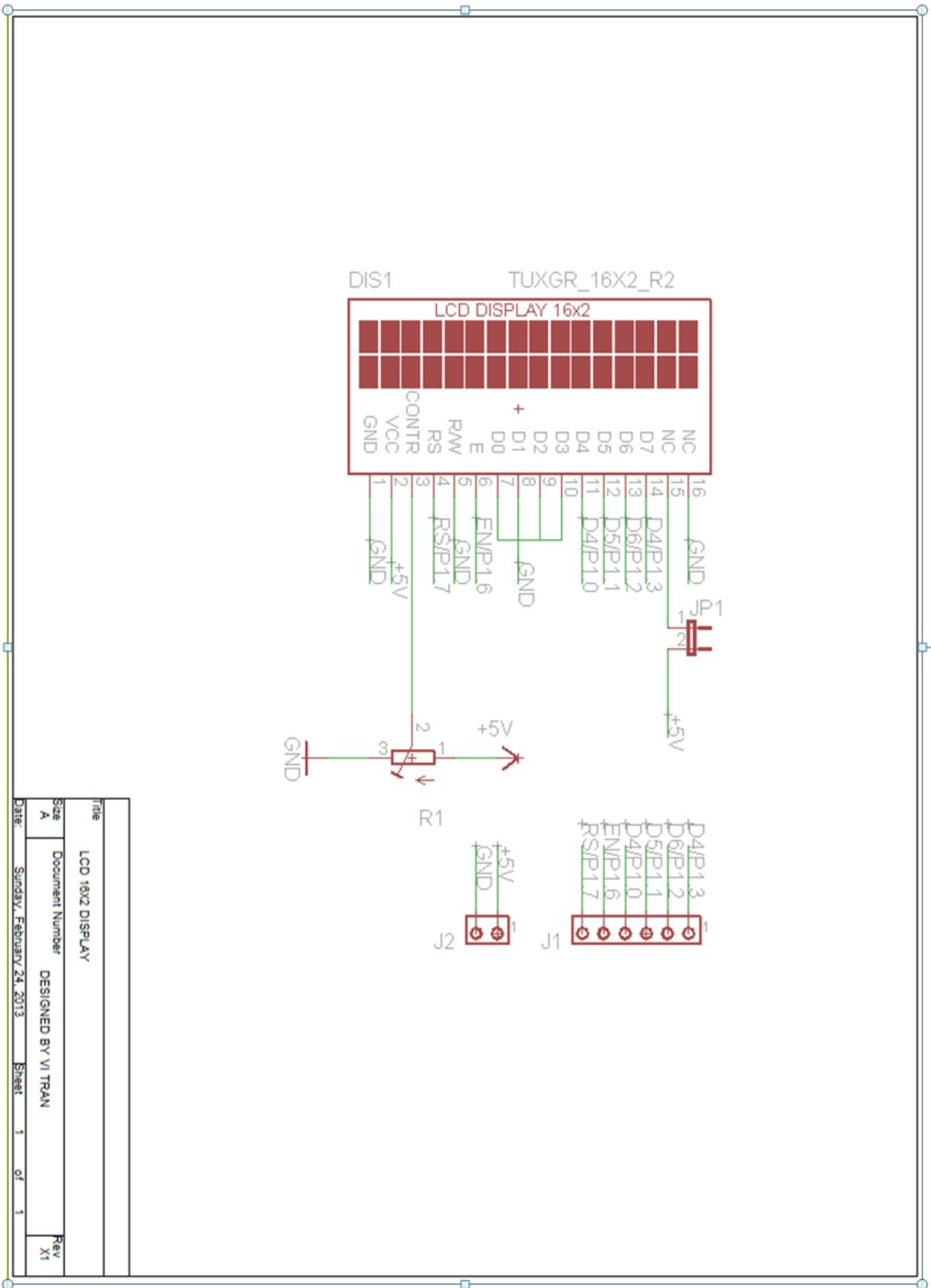
Figure 7: Liquid crystal display diagram
