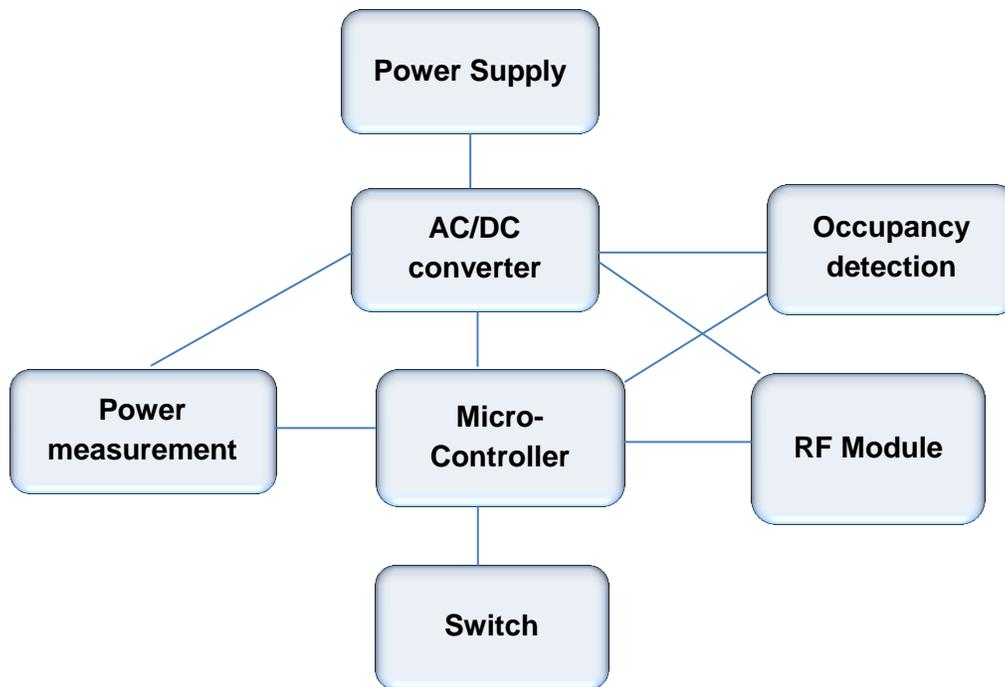
Figure 3: Block Diagram for Sensor Units
