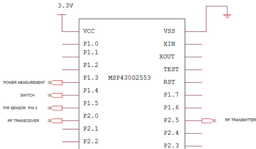
Figure 9.2: Microcontroller connection pin for the sensor units
