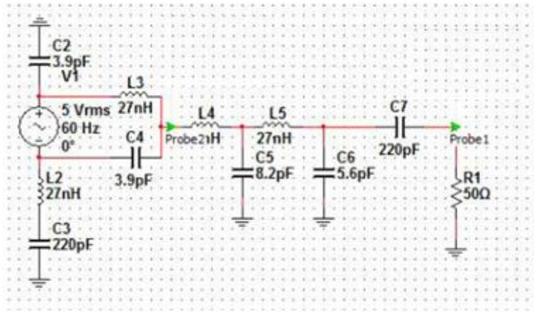
Figure 21: low pass filter circuit diagram
