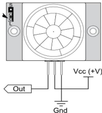
Figure 16: Basic Wiring<sup>3</sup>
