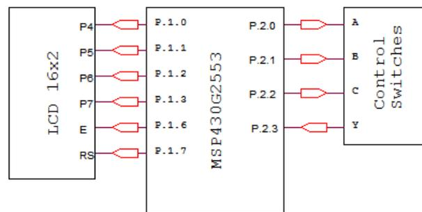
Figure 6: User I/O Pin with MSP430 microcontroller connection
