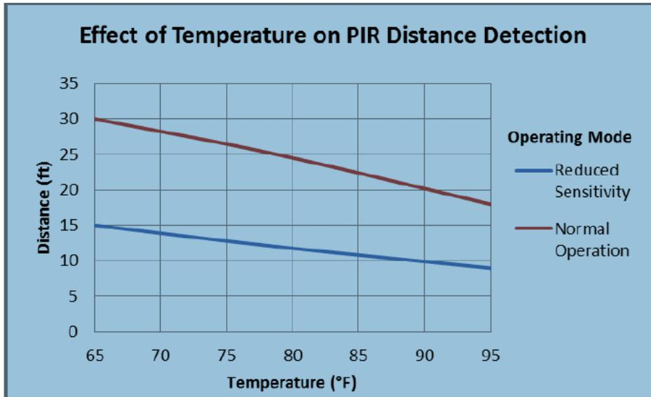
Figure 19: Effect of temperature on PIR distance detection<sup>3</sup>
