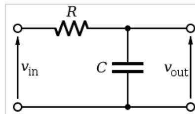
Figure 23: a low pass RC filter <sup>5</sup>
