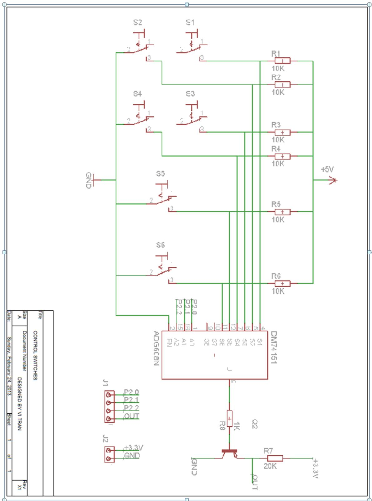
Figure 8: Push Buttons diagram
