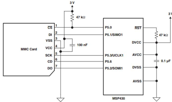
Figure 24 Connection between MSP430 and MMC card<sup>1</sup>
