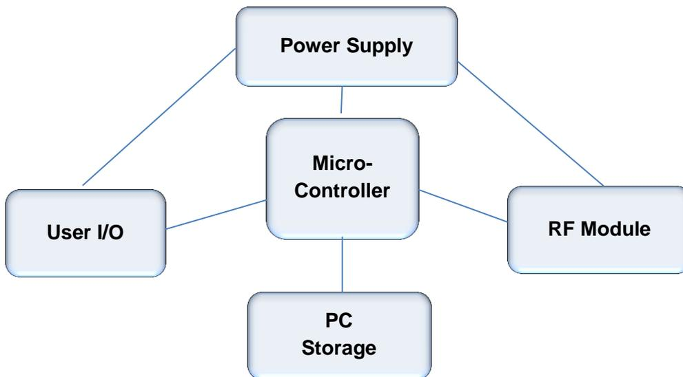
Figure 2: Block Diagram of Controller Unit
