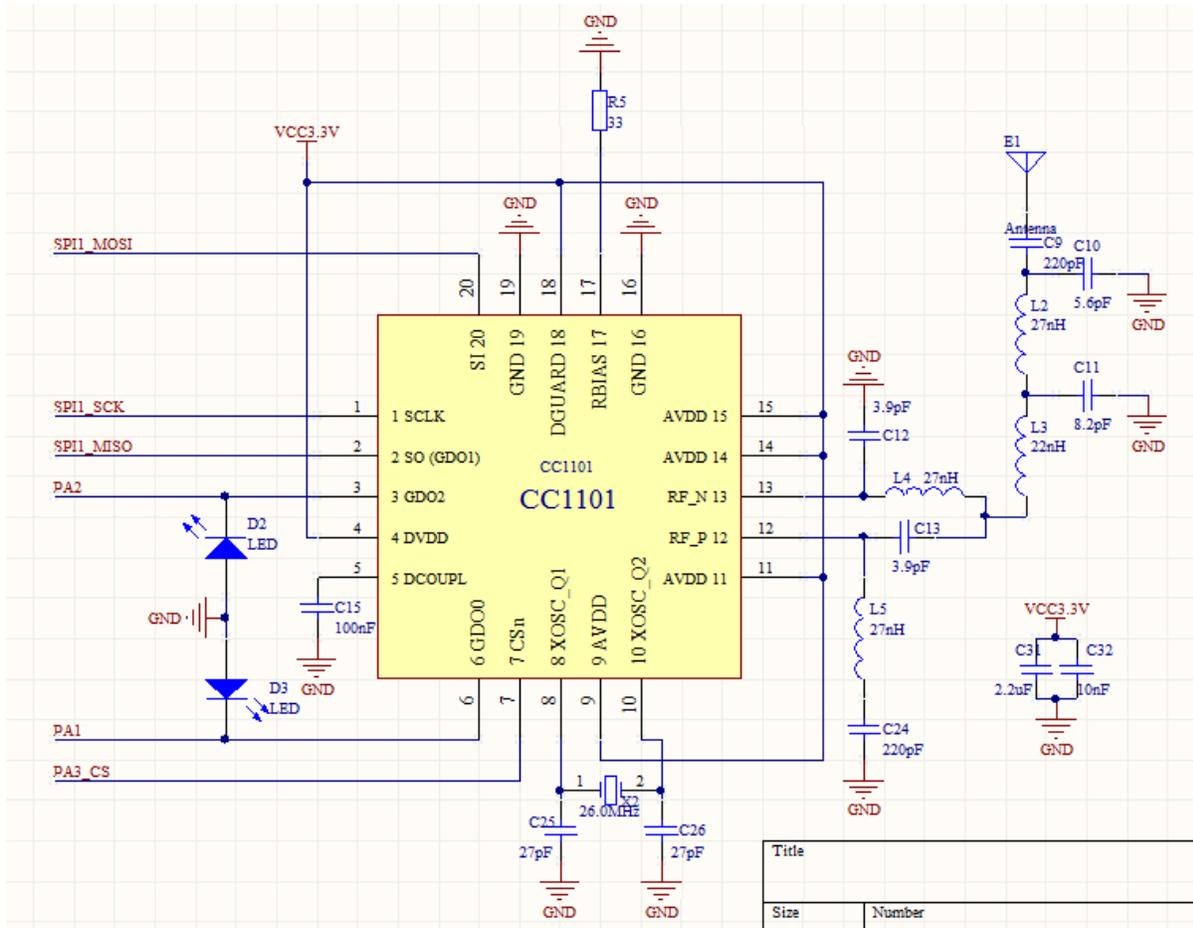
Figure 20: RF transceiver circuit diagram <sup>4</sup>
