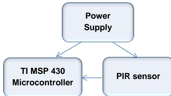
Figure 15: Motion detection flow chart
