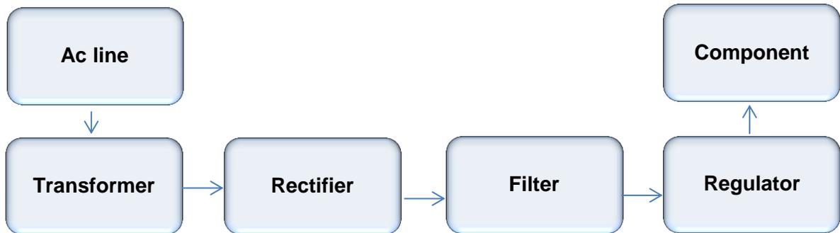
Figure 11: AC/DC converter flow chart
