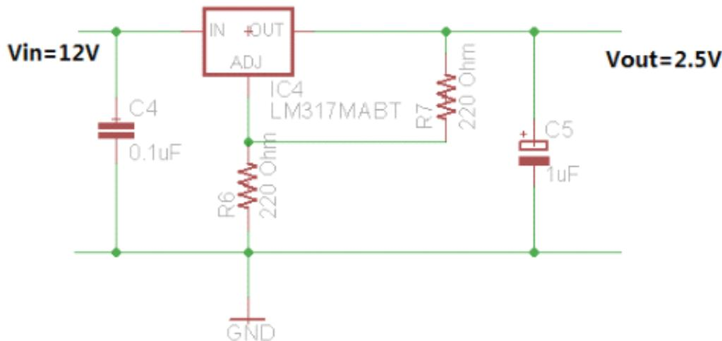
? 2.5V keeps dropping down while connected to the nichrome wire
