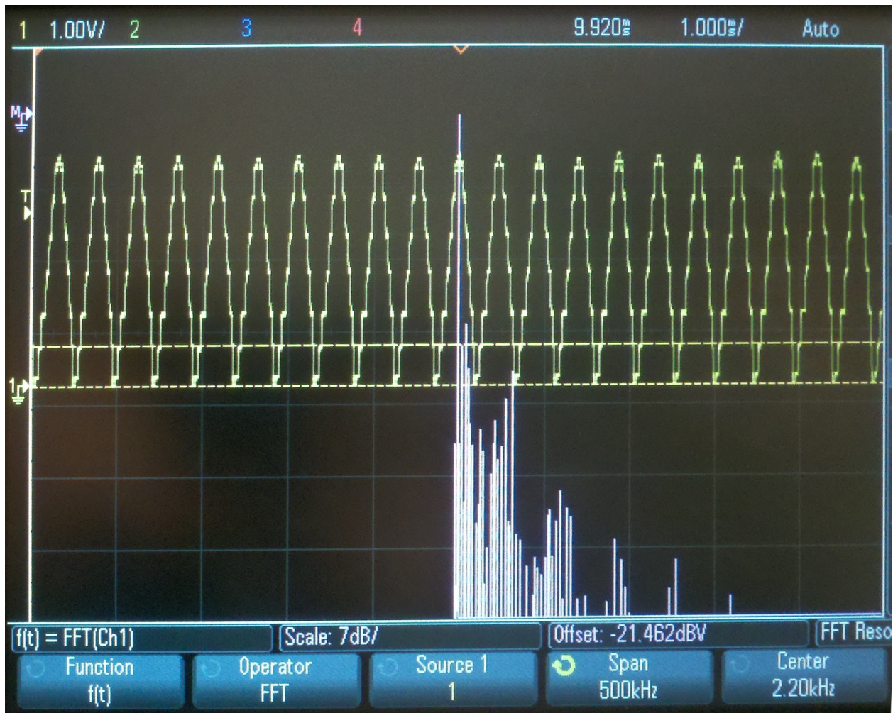
Figure 4: A sample 2.2kHz output sinusoid from the PIC16 DAC.
