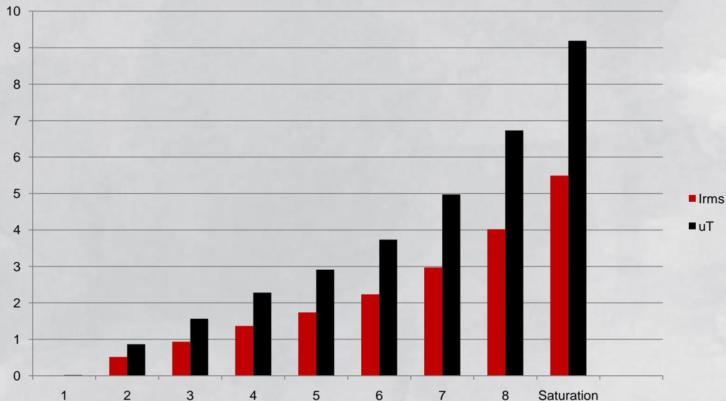
Chart shows input current and corresponding magnetic field levels, and the number of micro-transducers turned on
